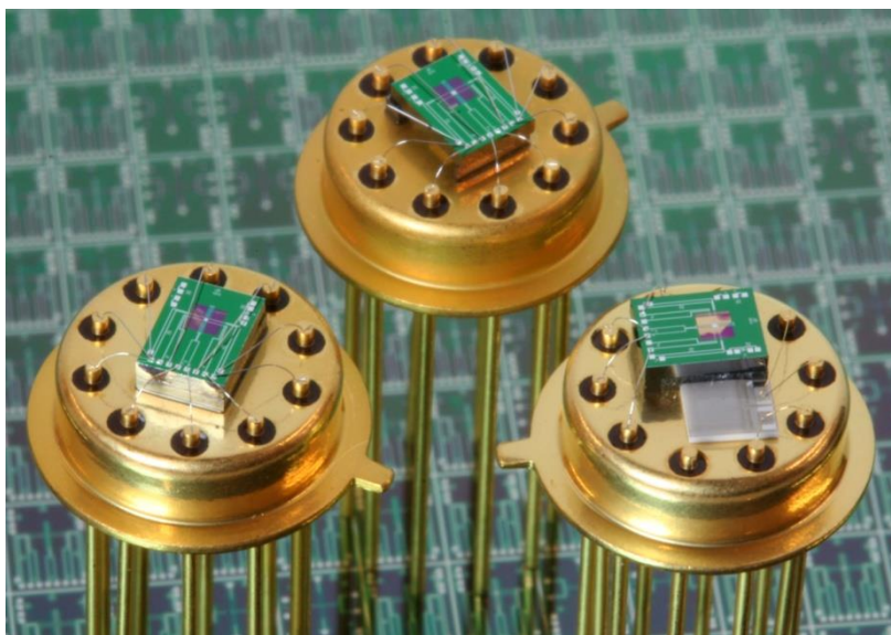
close up of nanogascalorimeter chips on TO-5 header
